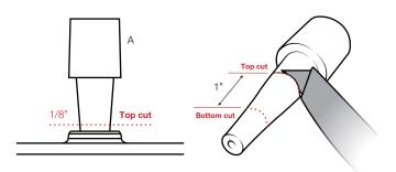
Assemble components as shown before using appropriate (E) Washer and (F) Nut Pocket Washer. Diameter of selected (E) Washer must not be wider than diameter of the top cut of (A) Expansion Plug. Tighten assembly until (F) Nut Pocket Washer has a firm grip on (A) Expansion Plug.
