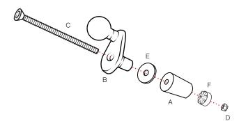
Insert assembly into fork stem hole until ball plate is flush with your bike. Tighten (C) Screw using a 3mm allen wrench. Periodically check the friction of the assembly to ensure it is tightening properly. If your assembly is not tightening, the (F) Nut Pocket Washer may not be gripping on the expansion plug. Remove assembly from hole and pre-tighten further, then repeat.
