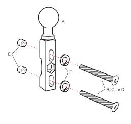
While holding factory clamp assembly in place, remove second factory bolt and replace with RAM® Base with hardware from Step 1. Store any unused components or hardware for possible future use.
