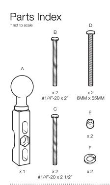
Preassemble components as shown below.
