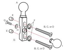
While holding factory clamp assembly in place, remove second factory bolt and replace with RAM® Base with hardware from Step 1. Store any unused components or hardware for possible future use.
