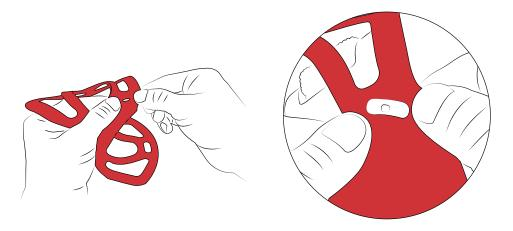
Wrap each of the four corners of (B) Tether around your tablet. Make minor adjustments to allow necessary access to camera, buttons and ports.
